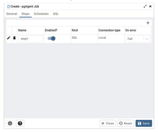
Use the *Steps* tab to define and manage the steps that the job will perform. Click the Add icon (+) to add a new step; then click the compose icon (located at the left side of the header) to open the step definition dialog:
