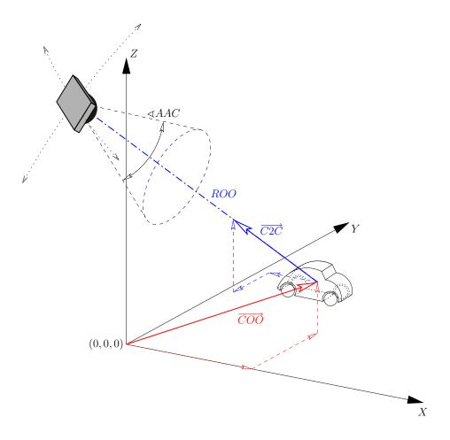
Figure 1: Camera and 3D object in the World System XYZ; centre of orbit position vector  $C\vec{O}O$ , centre of orbit to camera direction vector  $C\vec{2}C$ , radius of orbit ROO, aperture angle of camera  $\triangleleft AAC$ .
