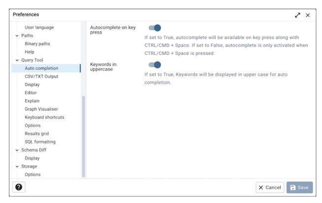
Use the fields on the Auto Completion panel to set the auto completion options.
