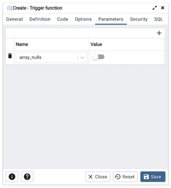
Use the fields in the *Parameters* tab to specify settings that will be applied when the trigger function is invoked. Click the *Add* icon (+) to add a *Name/Value* pair to the table below.
