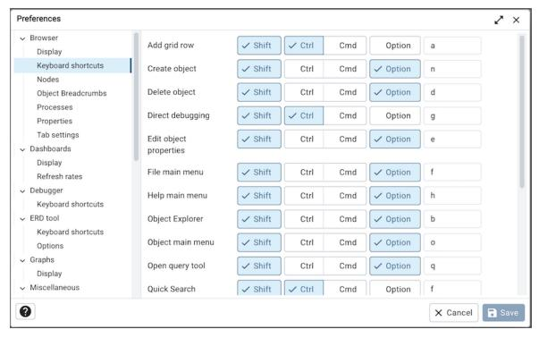
• The panel displays a list of keyboard shortcuts available for the main window; select the combination of the modifier keys along with the key to configure each shortcut.
