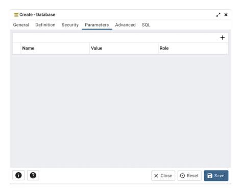
Use the *Parameters* tab to set parameters for the database. Click the *Add* icon (+) to add each parameter:
