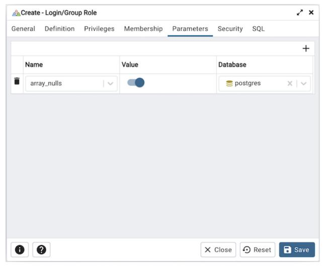
Use the fields on the *Parameters* tab to set session defaults for a selected configuration parameter when the role is connected to a specified database. This tab invokes the ALTER ROLE... SET configuration\_parameter syntax. Click the *Add* icon (+) to assign a value for a parameter.
