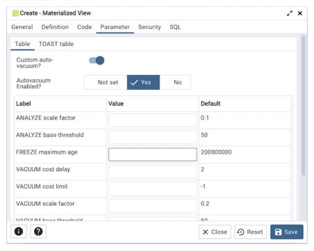
Use the tabs nested inside the *Parameter* tab to specify VACUUM and ANALYZE thresholds; use the *Table* tab and the *Toast Table* tab to customize values for the table and the associated toast table. To change the default values:
