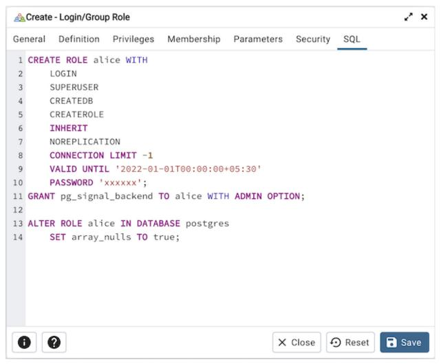
The example creates a login role named *alice* with *pg\_signal\_backend* privileges; the role can make unlimited connections to the server at any given time.
